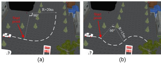
Fig. 8. Test scenarios. (a) a 90-degree bend with radius of curvature equal to 20m; (b) a S-Curve with radius of curvature equal to 15m. The white dash line is the designed track.
