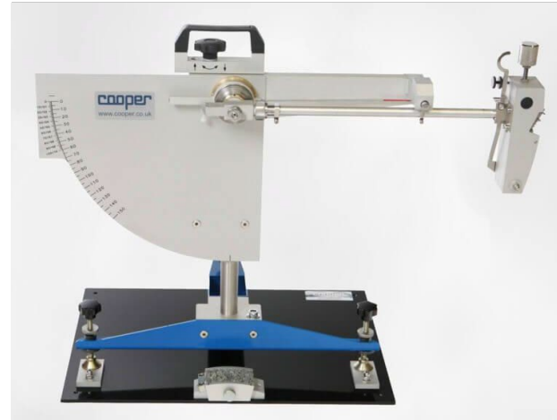
Cooper Pendulum Skid Resistance Tester
