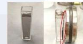
Figure 3. Separation of \text{CoFe}_2\text{O}_4/\text{TiO}_2 from the treated SMX solution.
