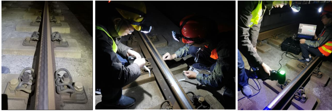
Figure 2.18 Measurement of rail corrugation and wheel wear on Wenzhou S1 line (second test)
