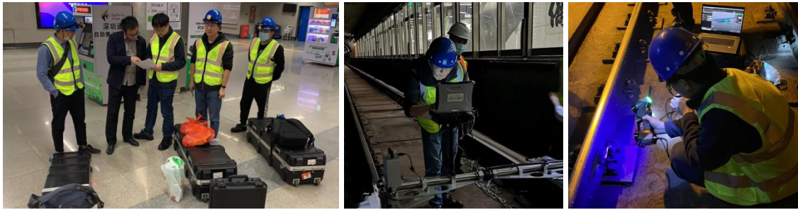
Figure 2.19 Measurement of rail corrugation on Shenzhen Metro curve line
