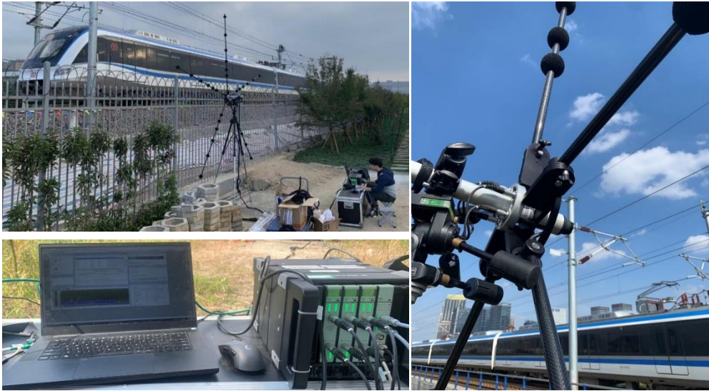
Figure 2. 13 Source/frequency resolving analysis of Wenzhou S1 line in October 2020
