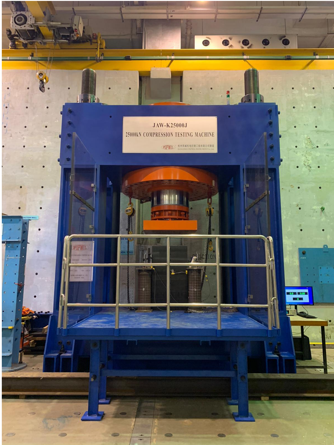
Figure 1 Prestressed main steel frame of the testing system
