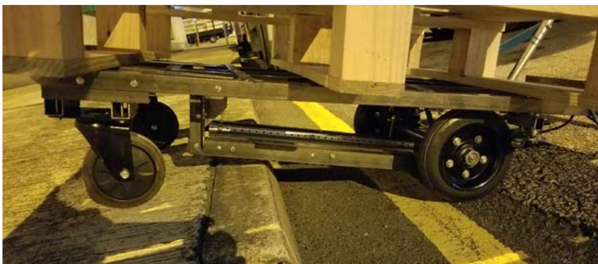
測試上壘的相片記錄 Documentation of kerb-climbing testing
