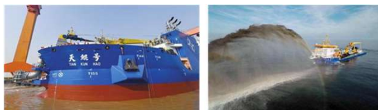
Figure 1: Tian Kun dredging and blow-filling ship
