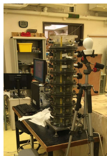
Smaller 2D cylinder model: 0.8m×0.17m (height × internal diameter)
