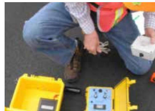
Moisture Sensor Measurement
