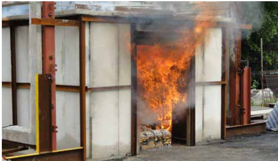
Full Scale Fire Burning Test for Heat Release Rate
