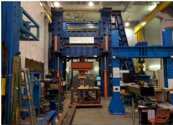
Testing of a strengthened column in Structural Engineering Laboratory
