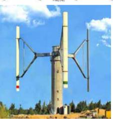
The straight-bladed vertical axis wind turbine (Courtesy of Hopewell Holdings Limited)
