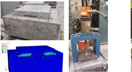
Fig.2 Anchorage capacity of the new stone façade system: laboratory tests and finite element analysis
