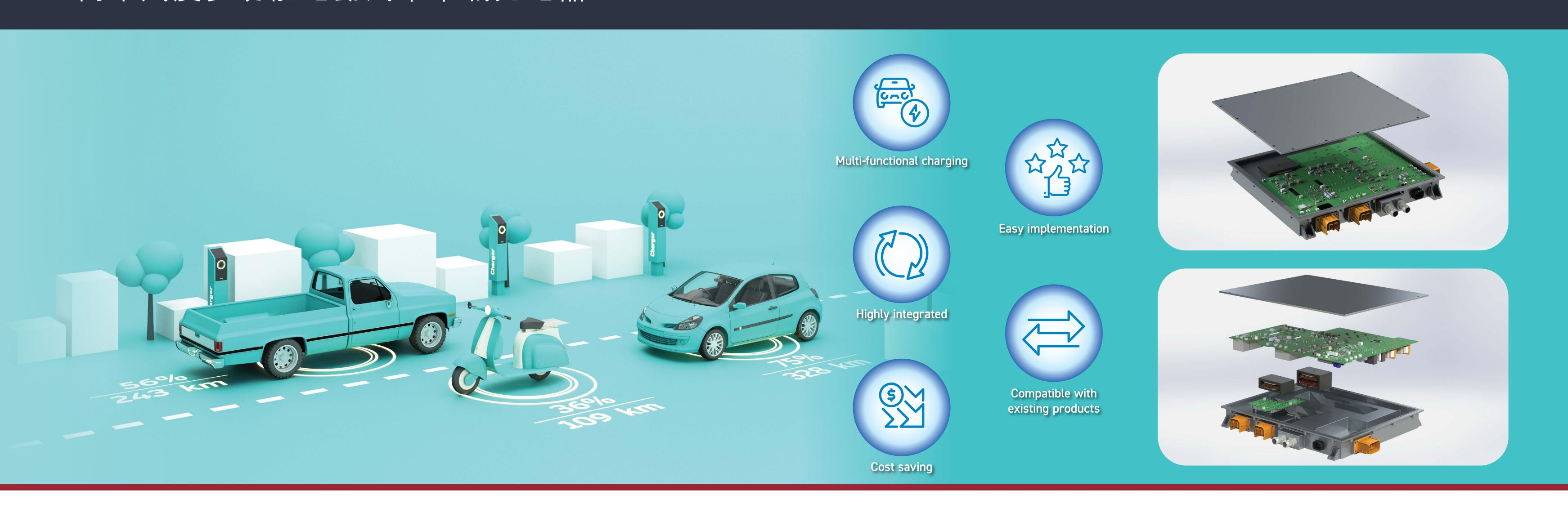
Electric vehicles are usually charged using conductive (plug-in) charging. However, wireless charging is becoming more popular and has many advantages. Future electric vehicles are expected to have both conductive and wireless chargers. Very few solutions currently combine both types of chargers. Those that do have disadvantages such as a large number of components, an inefficient conductive charger, or a slow charging time because it is not possible to energise both chargers at the same time.
