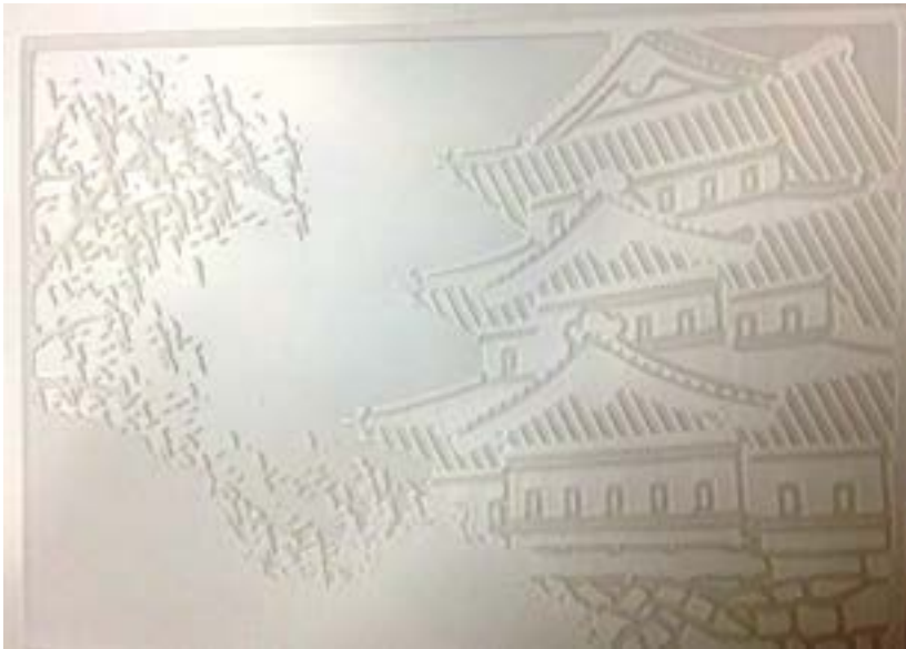
Figure 8: Second tactile diagram – ‘Thick pigment’ layer that provided a soft and embossed tactile surface.
