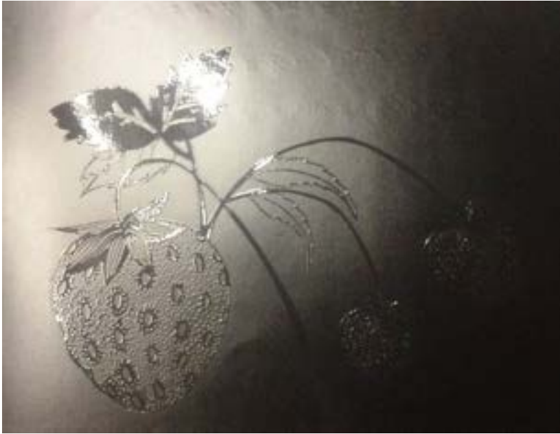
Figure 7: First tactile diagram – ‘Spot UV’ or ‘spot varnished’ printing technique that had a tactile effect.
