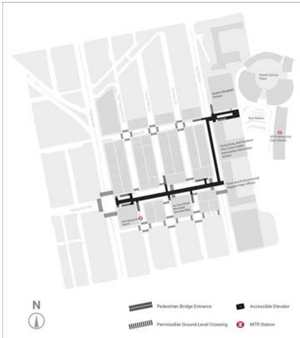
Figure 5-24 Pedestrians are guided by the limited access from Mong Kok Pedestrian Bridge to ground level and by the restricted permissible ground-level crossings.
