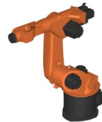
Fig.1 A schematic of 6-axis serial robot (KR 60HA, KUKA)
