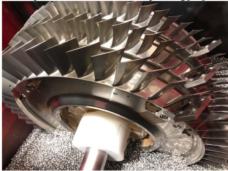
Fig. 2 Vibropeening of blisk drum setup with Almen blocks for process control (courtesy: Rolls-Royce)
