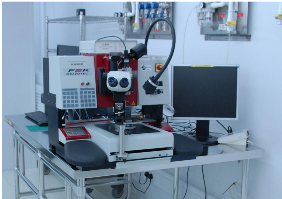
F&K Delvotec 5630 Semi-automatic Wire Bonder System
