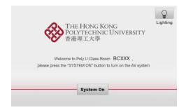
Press system on icon on the screen of control panel to turn on the AV system
