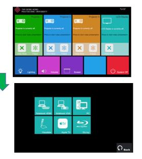
Press system on icon on the screen of control panel to turn on the AV system
